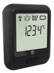
The EL-WiFi-TC in the EasyLog range of sensors measures the temperature of the environment in which the probe is situated. This sensor is typically accurate to ±1.5°C. Data is streamed wirelessly over any WiFi network and can be viewed on a PC or the EasyLog Cloud using the free software package.
